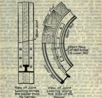
Fig. 4. Centers for Concrete Sewer.
